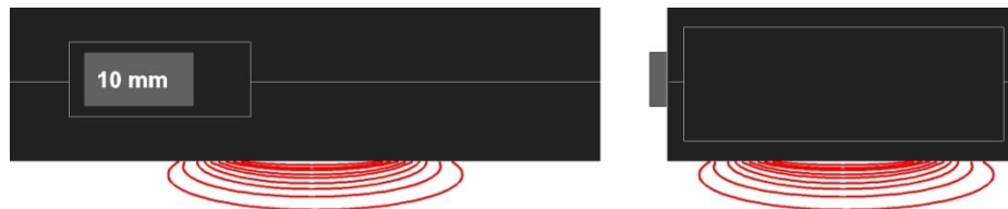
Side view: measuring field and penetration depth for switch setting "10 mm"
