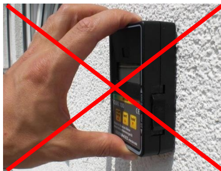
False: unsteady surface
