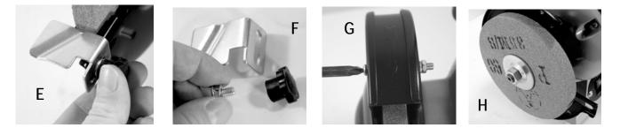
There is a left and right tool rest. When in actual use, the tool rests should be adjusted to within 1/8" (3.2mm) of the grinding wheel or other accessory being used. Follow the illustrations to remove/install the tool rest. The Grinding Wheel is accessed by removing the Eye Shield and Tool Rest and the Wheel Guard.
