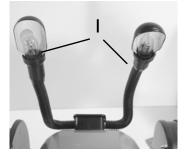
Your Bench Grinder may include adjustable lights. Lights can provide visual aid when using the Bench Grinder (Figure I) Note: You may choose to fasten the Bench Grinder to a secure base. The base includes predrilled holes to attach 5/16" bolts to a secure surface.
