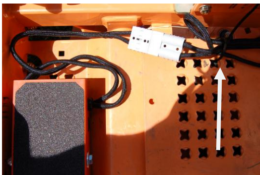
Proper mounting Wires tied down
