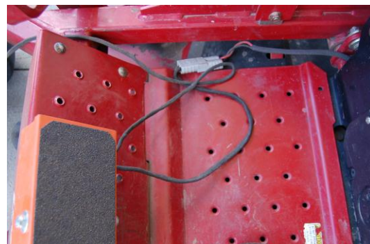
Improper mounting Wires not tied down
