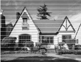
When an ink head nozzle is clogged the printed sample looks like this.
