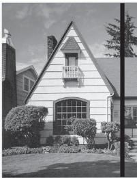
When there is a spot of dirt or correction fluid on the glass strip the printed sample shows a vertical line.
