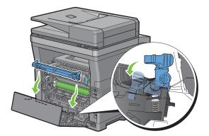
4 Make sure that the arrow marks on the transfer unit and the printer face each other, and then press the two tabs on transfer unit inward to lock.
