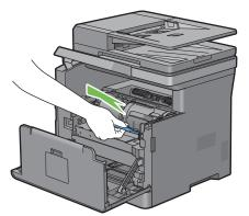
**3** Hold both sides of the drum cartridge with your hands, and then pull it out completely.
