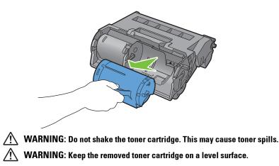
6 Install the removed toner cartridge to the new drum cartridge in the printer. Make sure that the two tabs of the toner cartridge align with the grooves on the printer, and then insert it into the printer until it clicks into place.
