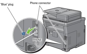
**3** To connect a telephone and/or answering machine to your printer, connect the telephone or answering machine line cord into the phone connector (<sup>PHONE</sup>).
