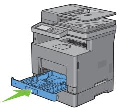
**11** Insert the MPF into the printer, push until it stops, and close the MPF cover.
