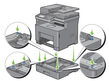
**9** Secure the optional 550-sheet feeder to the printer by tightening the two screws provided with the feeder, using a coin or similar object.
