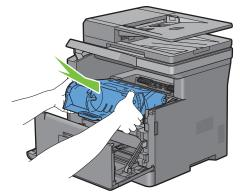
**3** Grasp the handle on the front of the drum cartridge, and then push and install the drum cartridge until it stops.
