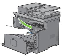
**4** To remove the toner cartridge from the old drum cartridge, grasp the toner cartridge lock lever, and then raise it upward to unlock.
