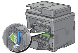
**3** Slide the envelope switches on both sides of the fusing unit to the **i** position.
