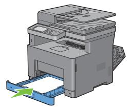
8 Insert the MPF into the printer, push until it stops, and close the MPF.
