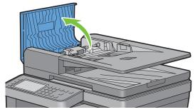
**b** Lift the release lever 90 degrees and remove the jammed document by carefully pulling it to the right.
