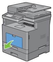
3 Grasp both sides of the MPF, and then pull the MPF from the printer.
