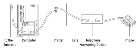
If you want to use your computer modem for faxing or for a dial-up Internet connection, connect the computer modem directly to the rear of your printer with the TAD as shown above.
