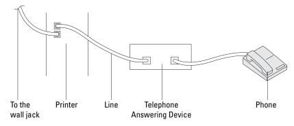
You can connect a telephone answering device (TAD) directly to the rear of your printer as shown above.
