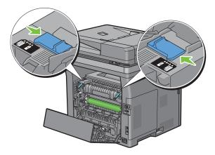
4 Press down the levers on both sides of the fusing unit.
