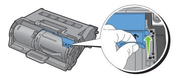
**5** Grasp the handle on the toner cartridge, and then pull it out of the old drum cartridge.
