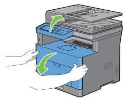
2 Grasp the toner cartridge lock lever, and then raise it upward to unlock.
