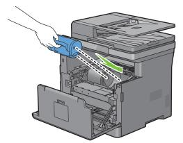
7 Grasp the toner cartridge lock lever, and then pull it down until it stops.
