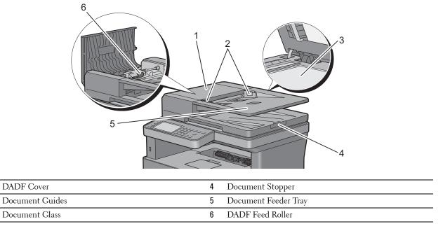
**NOTE:** Pull out the document stopper to prevent the document from falling off the printer.
