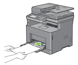
4 Slide both width guides until they rest lightly against the edge of the print media stack.
