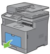
**5** Grasp both sides of the MPF, and then pull the MPF from the printer.
