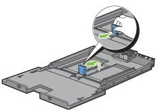
**5** Load the print media into the MPF with the recommended print side facing up so that the top edge of the print media enters the printer first.
