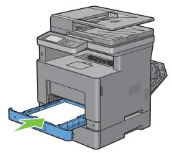
**11** Insert the MPF into the printer, push until it stops, and close the MPF.
