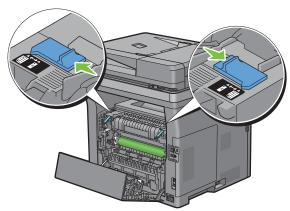
4 Press down the levers on both sides of the fusing unit.
