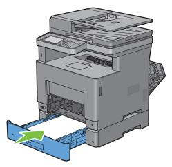
**10** Insert trayl into the printer, and push until it stops.
