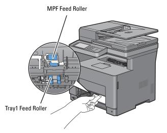
7 Insert trayl into the printer, and push until it stops.
