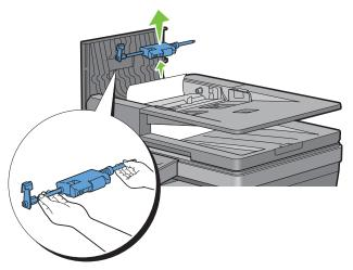
**d** Insert the DADF feed roller assembly and press down the release lever.
