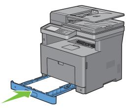
**NOTE:** If the front side of the tray is extended, the tray protrudes when it is inserted into the printer.
