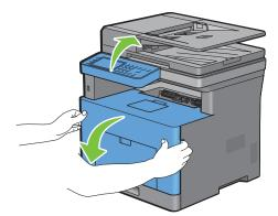
2 Grasp the handle on the front of the drum cartridge, and then pull it out halfway with one hand.
