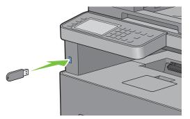
CAUTION: If you remove the USB memory while the printer is accessing, the data in the USB memory or the USB memory device itself may be destroyed.
