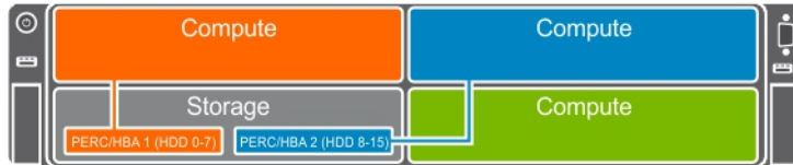
Figure 12. Split dual host configuration—four-bay chassis
