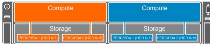
Figure 9. Split single host mapping configuration—four-bay chassis
