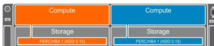
Figure 5. Single PERC/HBA joined mode mapping configuration—four-bay chassis
