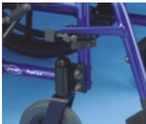
Precision head tube bearings allow casters to turn smoothly.
