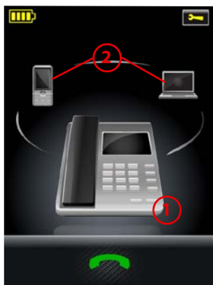
Figure 32: The current target phone is indicated by the large icon on the touchscreen; change the target by touching on one of the other icons.
