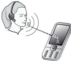
Figure 35: To use voice-activated dialing, tap the multifunction button and speak the appropriate voice tag.
