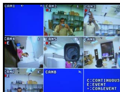
3x3 CHANNEL VIEW – Press the VIEW button to display all channels and legend.
