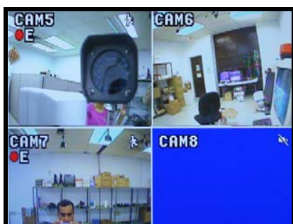
QUAD CHANNEL VIEW CAM 5-8 – Press the VIEW button to display the Quad View.
