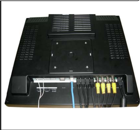
DEVICE CONNECTIONS (Stand Removed)
