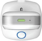
The indicator LED will glow **green** and flash on and off. After a few seconds, the LED steadily glows green. This means the camera is ready for remote connection.
