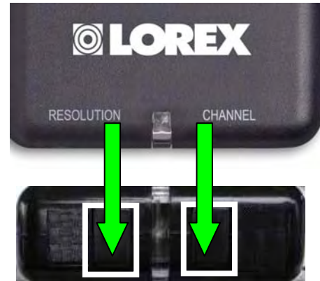
Figure 7.0 Press and hold the RESOLUTION and CHANNEL buttons at the same time
