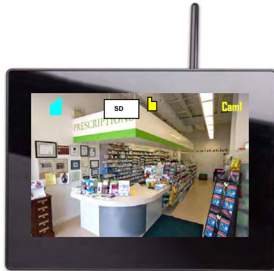
Figure 7.2 Schedule Recording on the receiver – "AUTO REC" must not appear in order for Schedule Record to function
