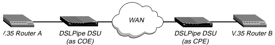
Figure 1-2. Example: Using a DSLPipe DSU as COE
