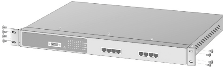
Figure 3-2. Attach mounting brackets with screws
