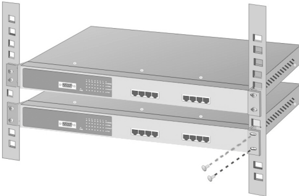
Figure 3-3. Mounting the MIL-S8000G in an EIA standard 19-inch Rack
