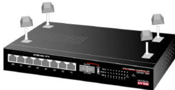
Figure 2-3. Attaching Rubber Feet to each corner on the bottom of the switch
