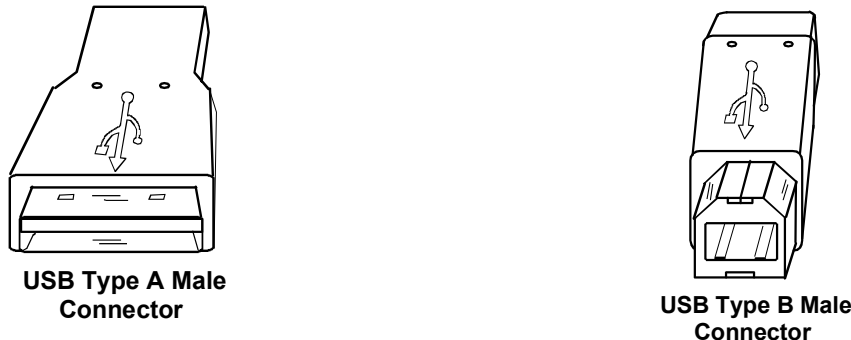
Figure 4- End views of USB Type A and USB Type B male connectors
