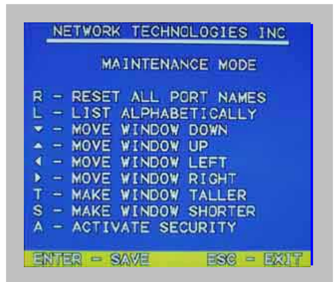
Figure 13- Maintenance Mode screen
