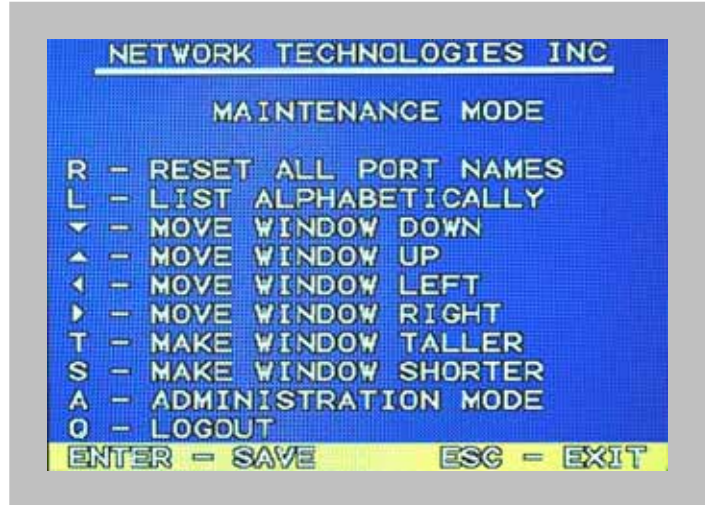
Figure 14- Maintenance Mode screen
