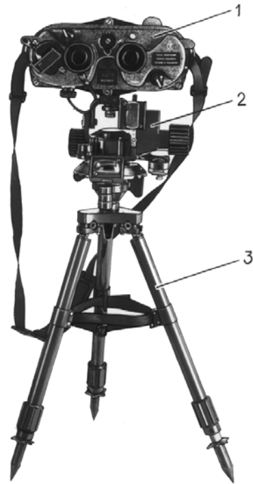
1 - range finder; 2 - Angular Mount; 3 - tripod Fig. 1
