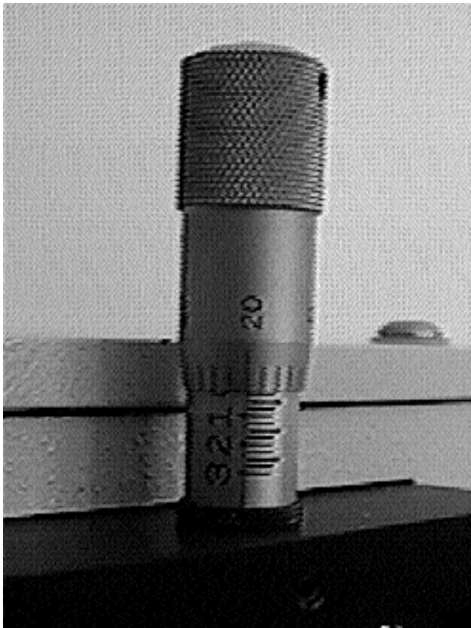
Slit Width Setting: 200 Micrometers (0.200mm)
