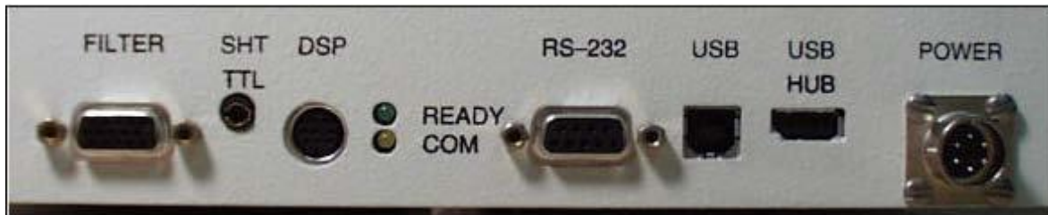
Figure 10. Cable Connections (Back Panel)
