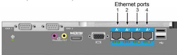
Figure 14: Ethernet ports on the rear panel of the Vess A2600
