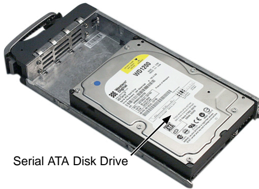
Figure 12. SATA Disk Drives mount at the front of the carrier
