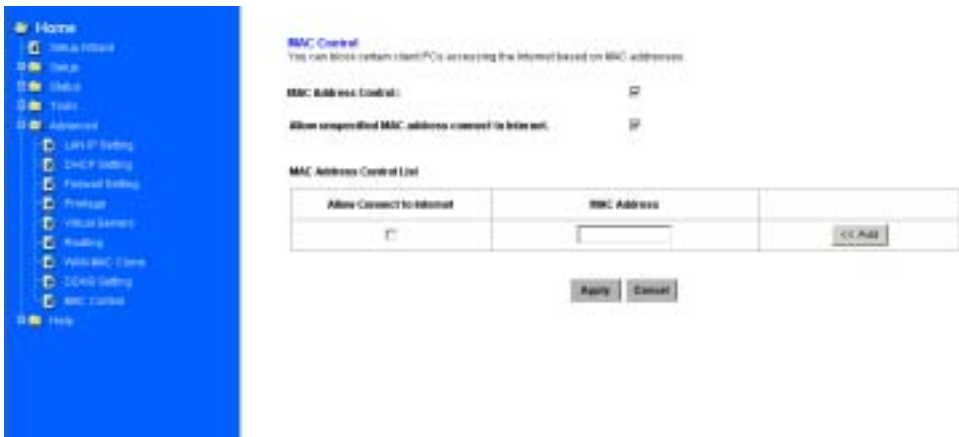
Figure 6-10: MAC Access Control Screen
