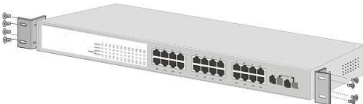
Figure 2-3 Attaching the brackets to the Switch
