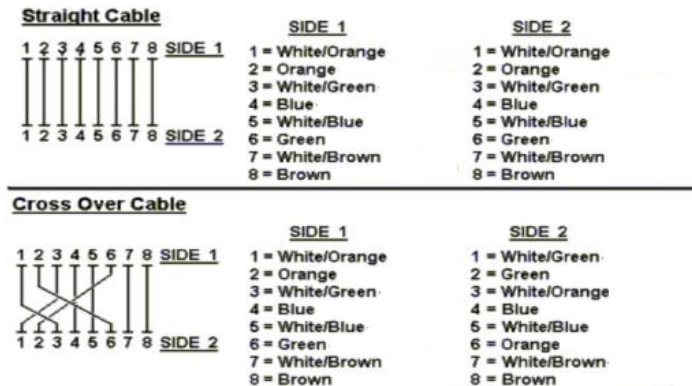
Figure A-1: Straight-Through and Crossover Cable
