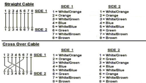
Figure A-1 Straight-Through and Crossover Cable
