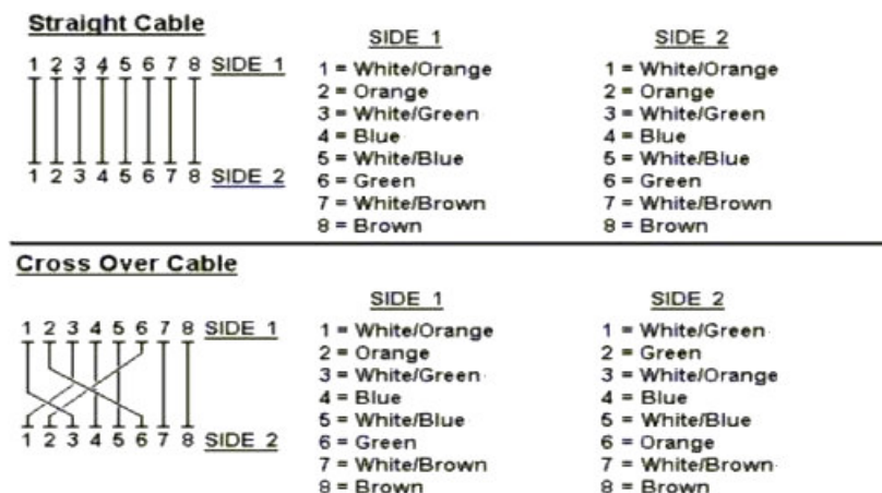
Figure A-1: Straight-Through and Crossover Cable
