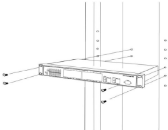
FIGURE 2-8 LOCATING A MOUNTING BRACKET
