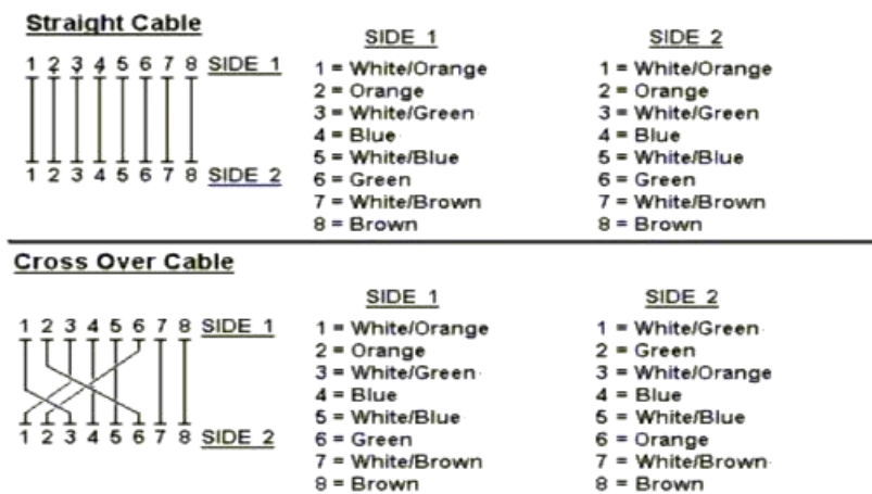
Figure A-1: Straight-Through and Crossover Cable
