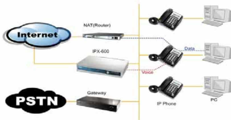
Figure 27. The installation environment of IPX-600 (IPX-600 used as an IP PBX only)
