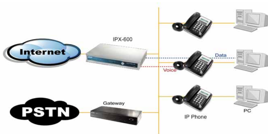
Figure 28. IPX-600 used as both IP PBX and NAT/Router
