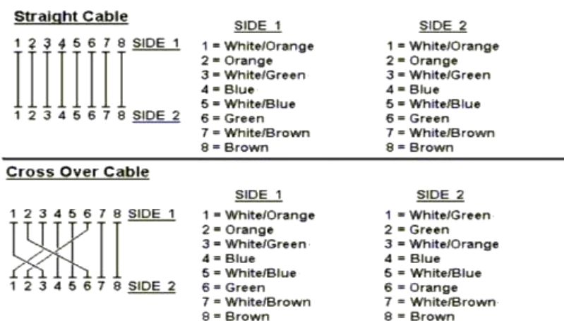
Figure A-1: Straight-Through and Crossover Cable
