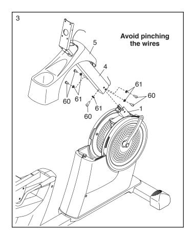
4. Locate the wire tie inside the Upright (4). Then, locate the Main Wire (76) and the Frame Pulse Wire (75) inside the Frame (1).
