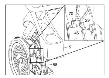
Locate the Reed Switch (46). Turn the Pulley (58) until a Magnet (29) is aligned with the Reed Switch. Next, loosen, but do not remove, the indicated M4 x 13mm Flange Screw (70). Slide the Reed Switch slightly closer to or away from the Magnet, and then retighten the Screw. Plug in the power adapter and turn the Pulley for a moment.
