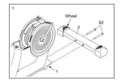
Set a sturdy piece of packing material under the rear of the Frame (1). Have a second person hold the Frame to prevent it from tipping while you complete this step.
