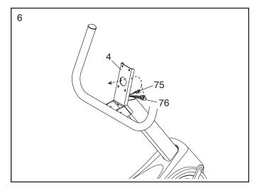
7. While a second person holds the Console (7) near the Upright (4), connect the wires on the Console to the Main Wire (76) and the Frame Pulse Wire (75).
