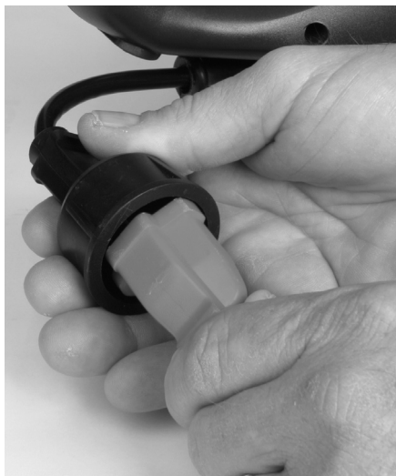
Figure 3-1: Plugging trimmer power cord into extension cord
