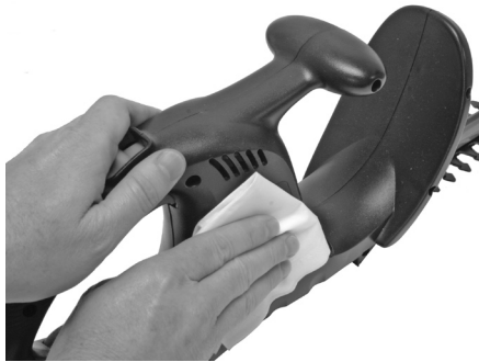
Figure 4-1: Cleaning trimmer housing
