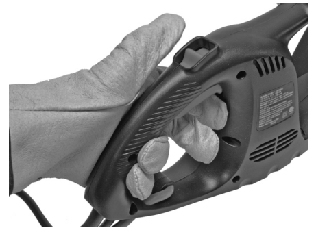
Figure 3-8: Releasing trigger switch to stop trimmer
