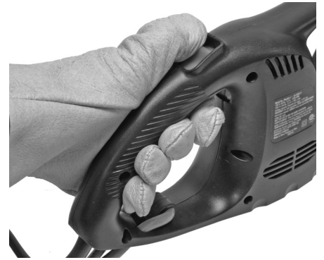
Figure 3-7: Squeezing trigger switch to start trimmer
