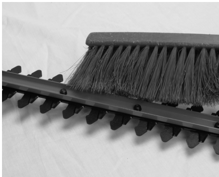
Figure 4-2: Cleaning cutter blades
