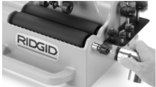
Figure 9 – Cleaning Inside of Fittings
