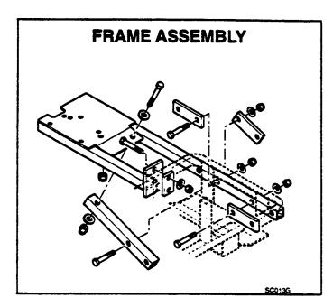
3/8-16 x 2.5" hex head bolts, flat washers and elastic stop nuts, along with two (2) rear tube clamps.
