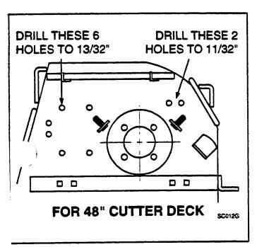
On the SSZ-48 using a 13/32" drill bit, drill the six (6) holes as indicated in the illustration. Using an 11/32" drill bit, drill the remaining two (2) holes.
