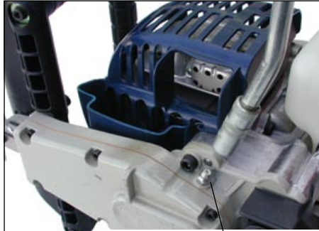
Figure 20 Gearcase Grease Fitting VIEWED FROM THE BOTTOM
