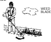
NOTE: If your unit has been assembled for trimmerheaduse, refertothesectionATTACH-ING THE PLASTIC SHIELD ANDTRIMMER HEAD and reverse the steps to remove the plastic shield and trimmer head before you mount the metal shield and blade. Storethese parts for future use. Neveruse that rimmerhead with the metal blade installed.
