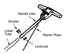
NOTE: When performing the following step, be sure the starter rope is not caught under the cable clamp. The starter rope must hang freely to operate properly.
