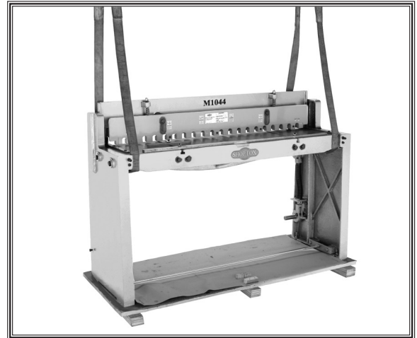
Figure 2. Lifting the foot shear.
