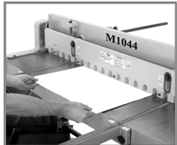
Figure 12. Paper shear test.
