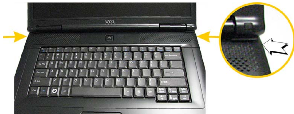
Figure 6 Prying off the switch cover
