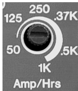
Figure 3-17 Equalize 2 Battery Capacity Rate Potentiometer (Position "0")
