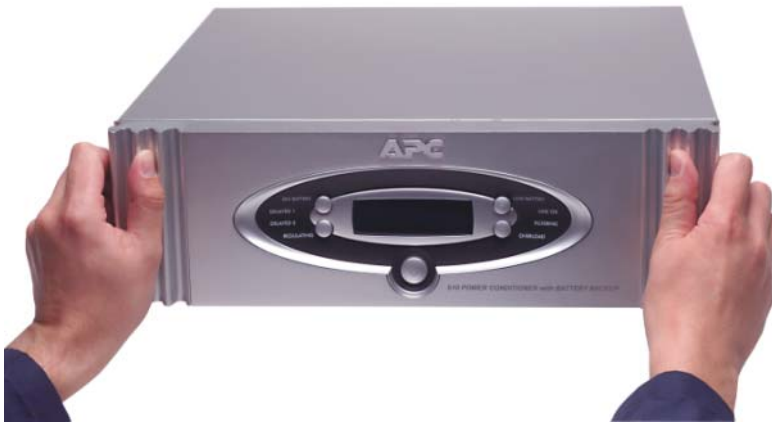
Figure 4. Front Bezel Removal
