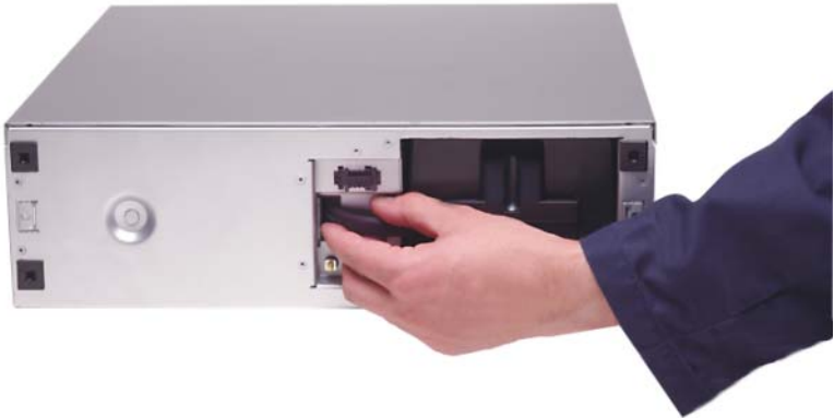
Figure 5. Battery Wire Connection
