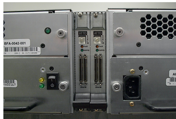
Exhibit 1.0-1 Back of rack mount model, Diamond Storage Array. Left: 2 gigabit Fibre Channel. Right: SCSI.
