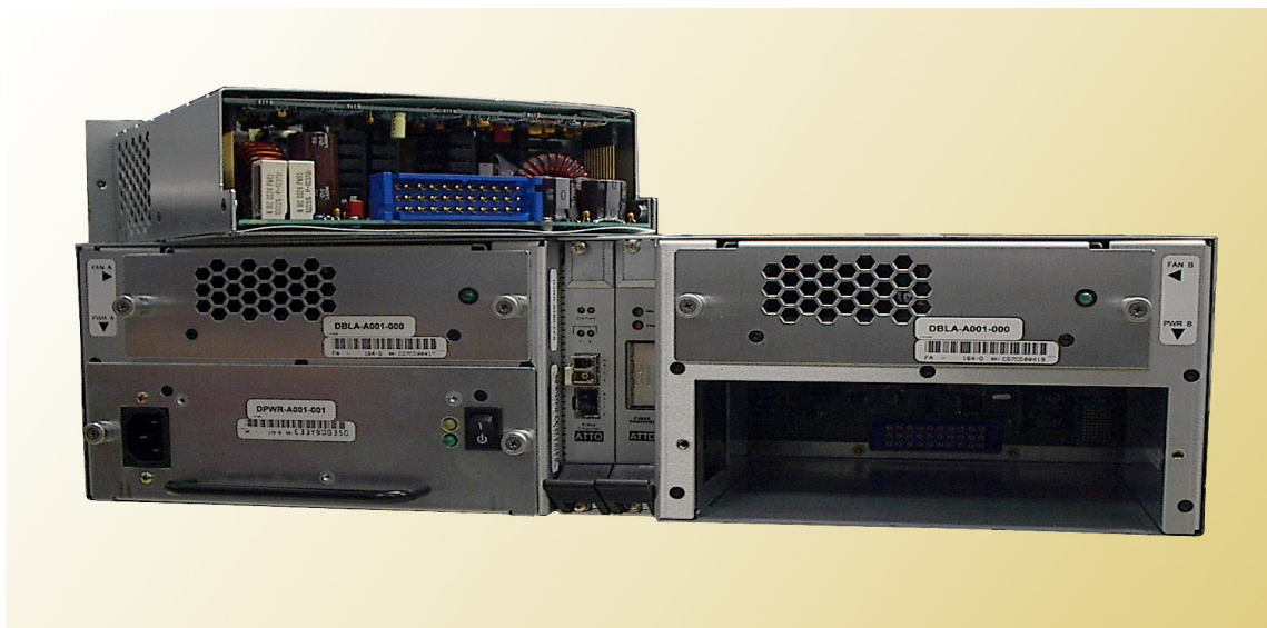
Exhibit 9-4: A power supply pulled out from a rackmount Diamond Storage Array: do not leave an empty opening while the Diamond Storage Array is operating. Access the blower assembly and the power supply by loosening the screws on either side of the component, then pulling out the part. If a blower or power supply stops working, keep it in place until another component is installed. (Note: host interface configuration pictured is not supported)
