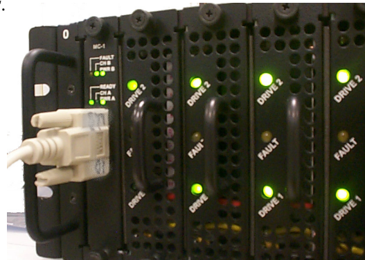
Exhibit 9-1: The management card may be accessed via a serial port DB-9 connector or an optional Ethernet connection.
