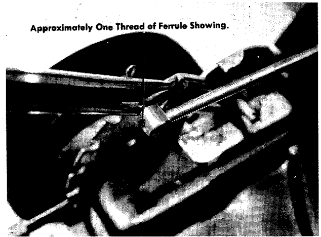
FIGURE F. CLUTCH ROD SETTING FOR THE SECOND LOWEST CUTTING HEIGHT
