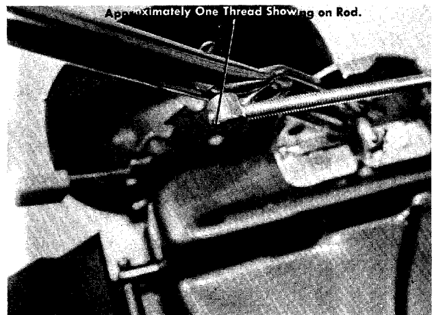
FIGURE G. CLUTCH ROD SETTING FOR THE LOWEST CUTTING HEIGHT.
