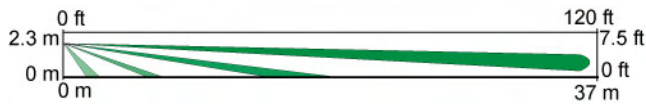
Side View Optional A120 Mirror Module: 37 m x 8 m (120 ft x 25 ft)
