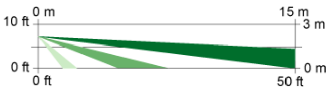
Side View Standard Broad Coverage 15 m x 15 m (50 ft x 50 ft)
