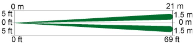
Top View Optional Long Range Coverage: 21 m x 3 m (70 ft x 10 ft)
