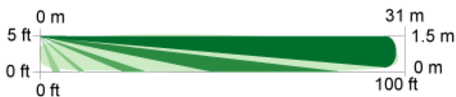
Side View Optional Long Range Coverage: 30.5 m x 3 m (100 ft x 10 ft) Requires optional ORL92-3 lens.
