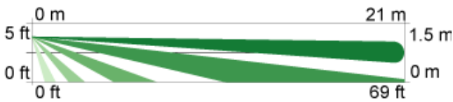
Side View Optional Long Range Coverage 21 m x 3 m Requires OMLR93-3 Long Range Mirror. Walking speed range is 0.2 m/s to 4.0 m/s.
