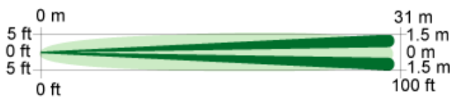
Top View Optional Long Range Coverage: 30.5 m x 3 m (100 ft x 10 ft) Requires optional ORL92-3 lens.
