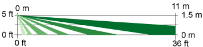
Side View Optional Barrier Coverage: 10 m x 3 m (35 ft x 10 ft)
