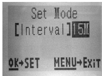
[Step 7]-set Field Scan Interval
