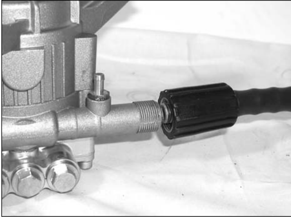
Figure 6 - Connect high pressure hose to pump
