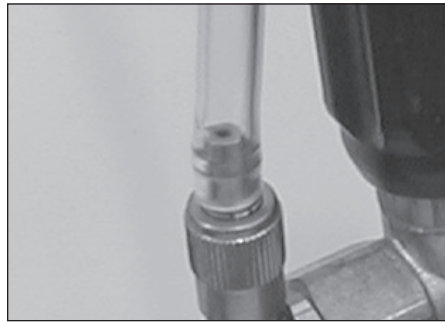
Figure 2 - Attach suction tube to barb fitting
