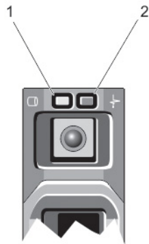
Figure 4. Rear SSD indicator patterns
